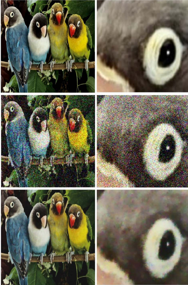
Fig. 4. The bird image denoising results. From top to bottom: the original image, the noisy image with \delta^2 = 0.04 , and the restored image by NKS algorithm. The whole image is shown on the left and a detailed partial image is on the right. Here \alpha = 0.3 , \beta = 10^{-4} , and PSNR=26.1205.
