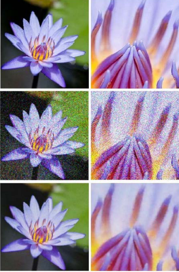
Fig. 2. The flower image denoising results. From top to bottom: the original image, the noisy image with \delta^2 = 0.04 , and the restored image by NKS algorithm. The whole image is shown on the left and a detailed partial image is on the right. Here \alpha = 0.3 , \beta = 10^{-4} , and PSNR = 27.2209 .
